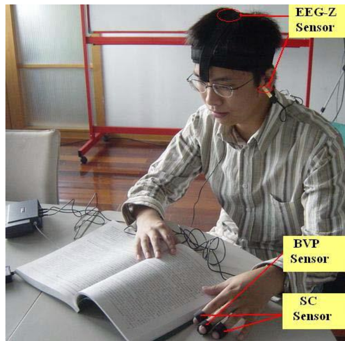
Figure 12: The Detection on the Relationship of Brainwave and Emotion by Thought Technologies ProComp 5 Suite.
